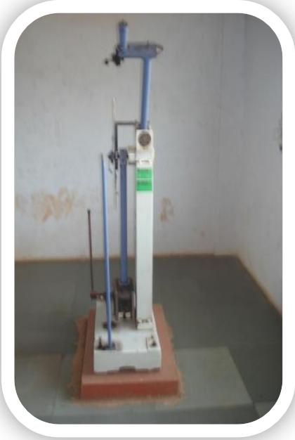
A photograph of a Charpy and Izod impact testing machine. The machine is tall and slender, with a blue frame and a white base. It has a vertical column with a pendulum arm at the top. The machine is placed on a wooden surface in a laboratory setting.                                        |
