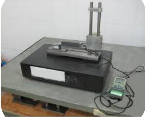
A photograph of a surface roughness tester. The device consists of a black base unit with a digital display on the front, and a vertical probe assembly mounted on top. The probe assembly includes a vertical column and a horizontal arm that holds the measuring stylus. The entire setup is placed on a grey table. A small digital display unit with a green screen is connected to the main device via a cable. |
