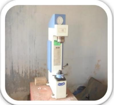
A photograph of a Rockwell and Brinell hardness testing machine. The machine is primarily white with blue accents on the top and sides. It features a vertical column with a dial at the top and a sample holder at the bottom. The machine is placed on a wooden surface in a laboratory setting. |
